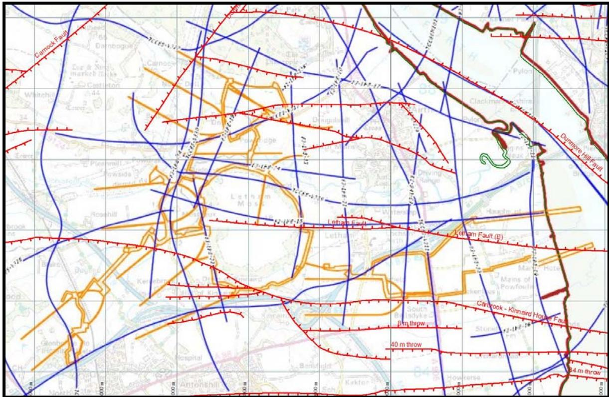
Fig. 1. Dart seismic database in relation to the PDA and surface-mapped faults.
