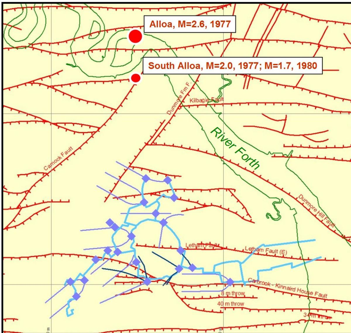
Figure 5. Epicentres of Alloa and South Alloa earthquakes (red circles) recorded between 1970 and the present. Faults at the surface are shown in red, with tick marks on the downthrown side. The proposed development is shown in shades of blue.
