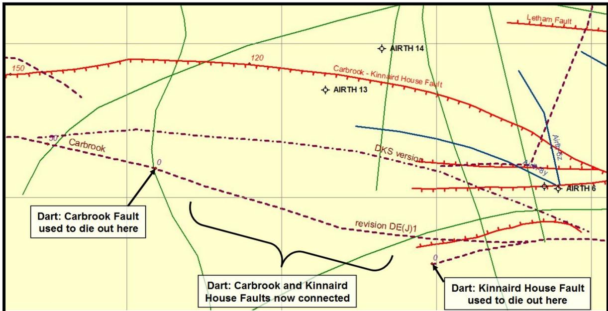
Fig. 2. Three interpretations of the Carbrook - Kinnaird House Fault at the depth of the coal horizons to be developed. These are (1) two separate faults (Dart, October 2013), (2) a continuous fault (Dart, January 2014, document DE(J)1), and (3) a more reasonably positioned continuous fault labelled 'DKS version'.
