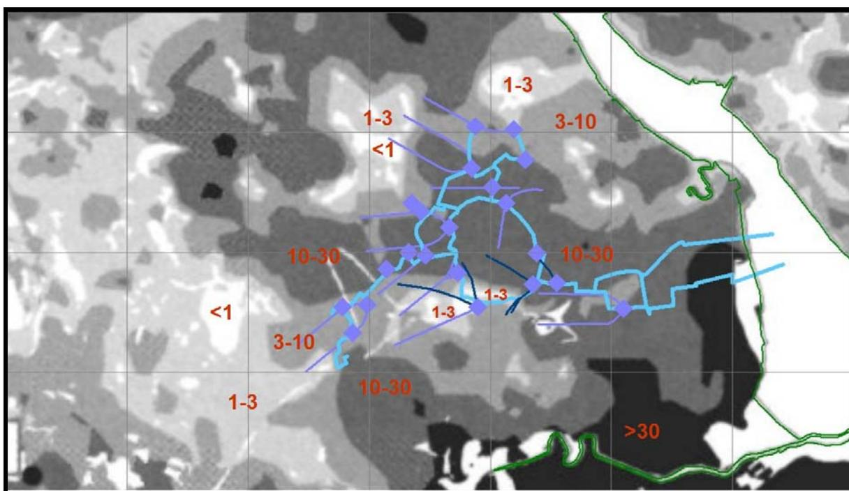
Fig. 4. Quaternary thickness in the PDA, in metres. Greater than 30 m - dark grey, with three progressively lighter shades as labelled in red. White - less than 1 m.
